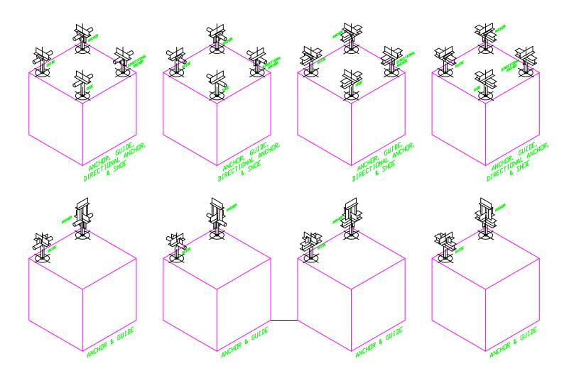
PS W/ PIPE SHOE, GUIDE, ANCHOR, DIRECTIONAL ANCHOR
